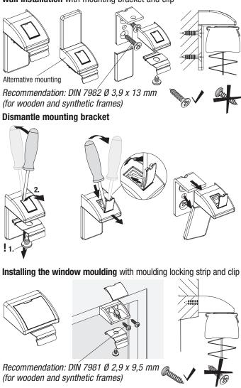
Mounting window frames with holding clamps
