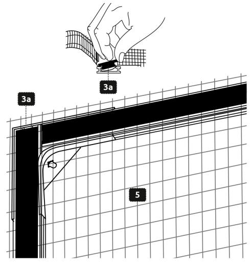
Shorten the material 5 on the outer side along the magnetic clamp 10 with a cutter.
