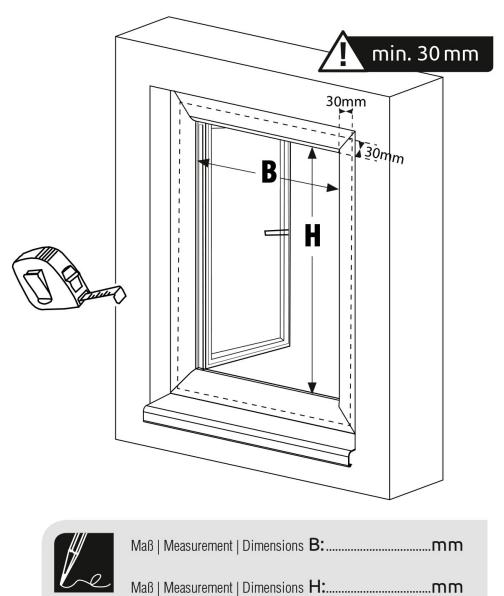
Mark both sections 1 and magnet strips 3 with measurement H plus 60 mm. Shorten both sections at the marked point with a metal saw. Example: Measured clearance height H = 1000 mm + 60 mm = 1060 mm. Attention: Risk of injury! Use the saw with caution.
