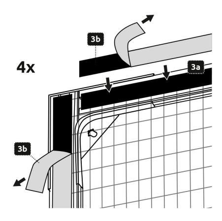
Glue the window evenly to the window frame. The grips 4a are located on the lower side of the window.
