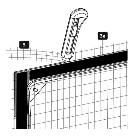
Attach the adhesive magnetic strips 3b to the clamps 3a and then remove the protective film.
