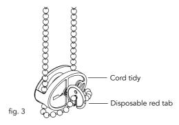
Remove the disposable red tab by disengaging it from the chain (fig. 4) and then pull out the disposable red tab (fig. 5).
