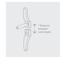
Mark the hole positions and drill as required.
