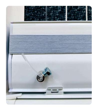
3.2 Fit the motor side of the Blind first to rail 'A1'. Start at one end and clip the motor side of the Blind into rail 'A1' as per the diagram and image below. We recommend resting the Blind on the side rails 'B1' and 'B2' whilst doing so. Begin clipping at one end and make your safely way across. Moderate force is required.
