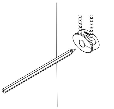
Split the cord tidy (fig. 7) and mark the remaining offset hole position (fig. 8) before drilling and plugging both location holes if necessary (fig. 9). Screw into the offset hole to fix the back piece of the cord tidy to the wall (fig. 10).
