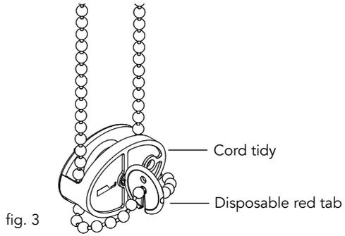
Remove the disposable red tab by disengaging it from the chain (fig. 4) and then pull out the disposable red tab (fig. 5).
