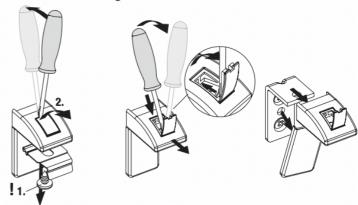
Installing the window moulding with moulding locking strip and clip
