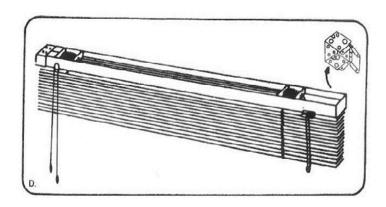
Attach a minimum of 2 plastic clips over the edge of the headrail & engage. DO NOT FIT VALANCE until blind is safely in place. Fit valance into clips.
