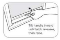
11) Release with care, holding the handle(s) or Pull-cord to be sure that the integral Brake mechanism is functioning. Try this several times to see that the screen returns gently into the Cassette.
