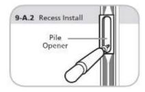
7) Insert the black plastic Pile Opener Tool (optional) into the Guide at a point where you will fix into the reveal, separating the strips of pile to clear access for drilling and screwing. This may require
