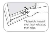
15) Release with care, holding the Handle(s) or Pull-cord to be sure that the integral Brake mechanism is functioning. Try this several times to see that the screen returns gently into the Cassette.
