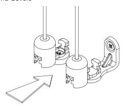
Place and align the base plate and cover into the end caps and mark the correct position where it has to be fixed - this could be face or base fixed. Remove the top cover and then fasten the base plate with a No 6 screw.
