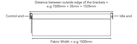
Use this figure to position the outside of your brackets accordingly whether inside of the recess or outside of the recess
